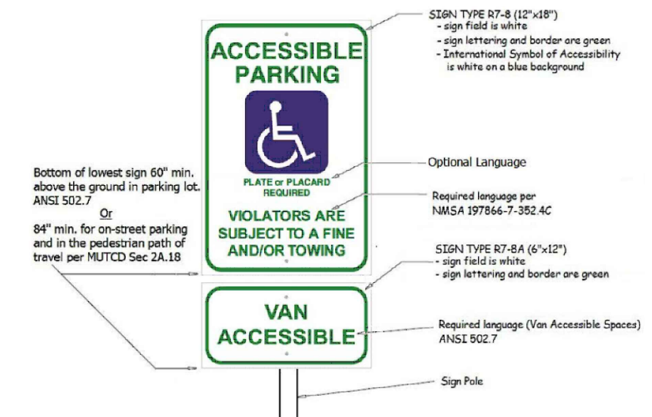
D6 RESERVED PARKING SIGNS NOT TO SCALE PROVIDE SIGN POSTS AND MOUNTING PER D3/C502.
